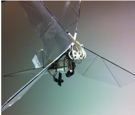
Figure 2: Photo of biplane-wing configuration of the DelFly II.
