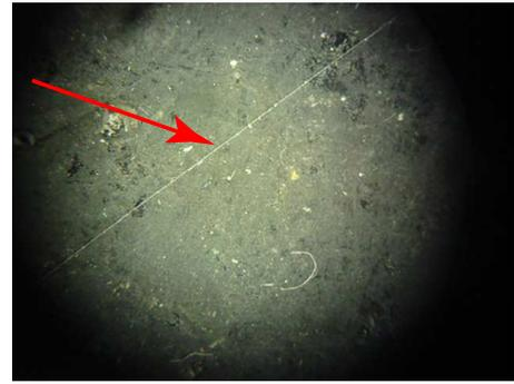
**Figure 6.15:** Microscopic view of a razor blade cut.
