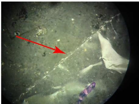
**Figure 6.12:** Microscopic view of an engraver cut with speed 12 mm/min.
