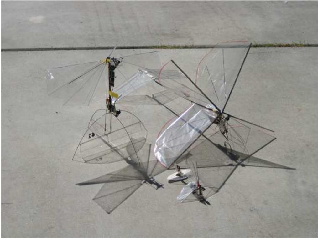
**Figure 2.4:** DelFly I (right), DelFly II (left) and DelFly Micro (middle).
