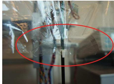
**Figure 5.26:** Rupture at the rear of the root.
