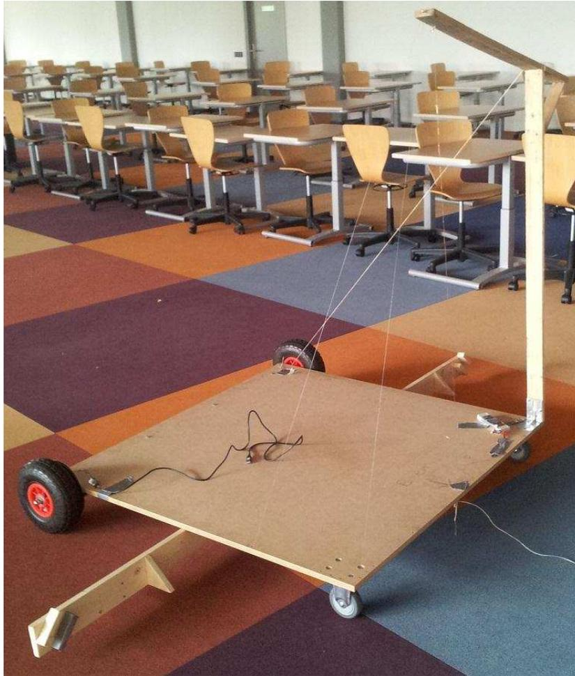
**Figure D-5:** The moving platform, showing the wooden support in front to attach the Delfly to by a safety tether. The larger back wheels accommodate the velocity tracking system
