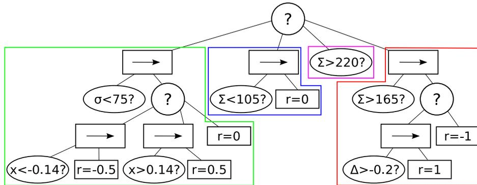
**Figure 5-4:** Graphical depiction of user-defined BT. Colours highlight different phases of the flight.  $x$  is the position of the centre of the window in frame,  $\sigma$  is window response value,  $\Sigma$  is sum of disparity and  $\Delta$  is the horizontal difference in disparity
