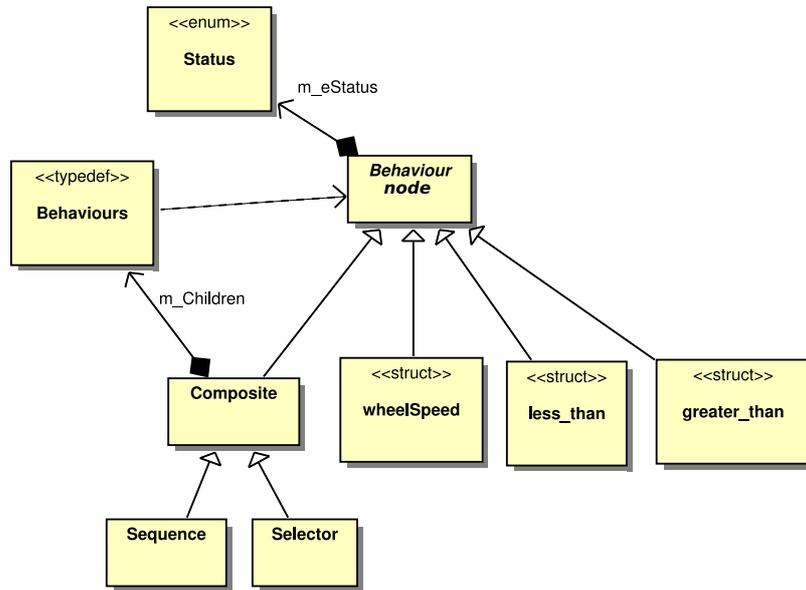
**Figure B-2:** UML class diagram of the Behaviour Tree framework for the wheeled robotic vehicle Khepera
