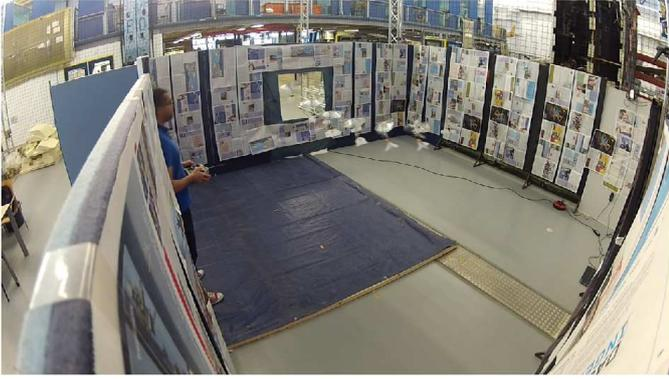
Fig. 12. Photograph showing the room environment used to test the DelFly Explorer for the fly-through-window task. Inset is collage of DelFly as it approaches and flies through window
