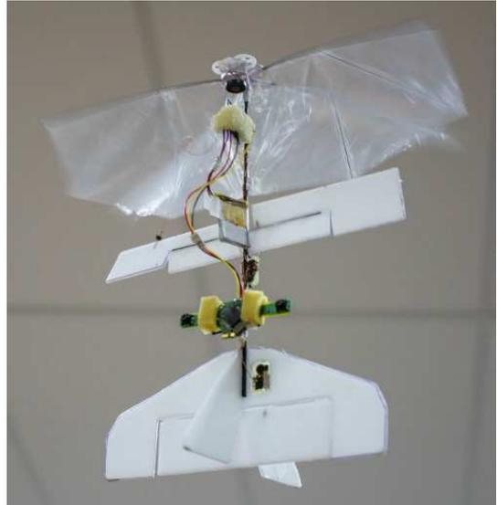
Fig. 1. DelFly Explorer in flight showing dual camera payload
