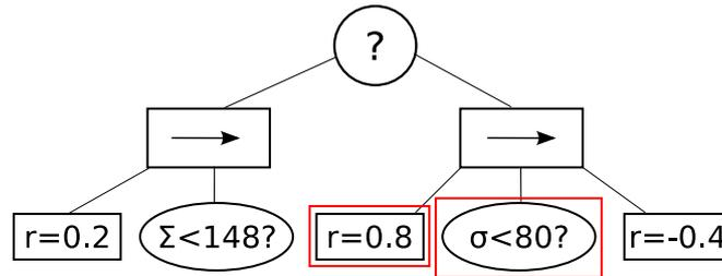
**Figure 6-3:** Graphical depiction of genetically optimised BT after modification for real world flight. Red boxes highlight updated nodes.  $x$  is the position of the centre of the window in frame,  $\sigma$  is window response value,  $\Sigma$  is sum of disparity and  $\Delta$  is the horizontal difference in disparity
