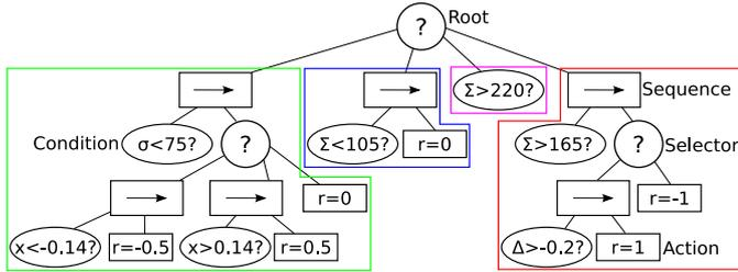
Fig. 2. Graphical depiction of user-defined BT for the fly-through-window task. Colours highlight different phases of the flight.  $x$  is the position of the centre of the window in frame,  $\sigma$  is window response value,  $\Sigma$  is sum of disparity and  $\Delta$  is the horizontal difference in disparity
