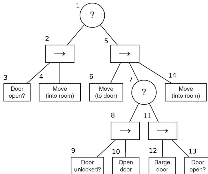
**Figure 2-3:** An example of BT used to define the behaviour to open a door Millington & Funge (2009) (modified for clarity)
