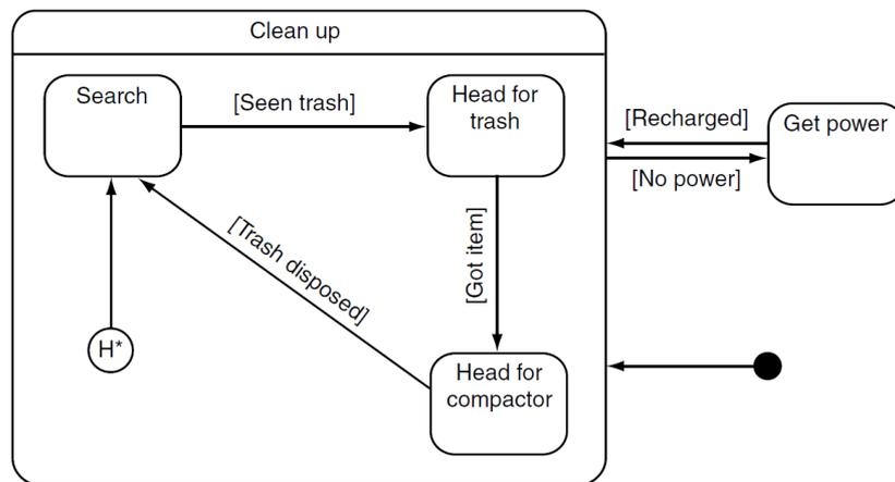
**Figure A-10:** Example of how HFSM can be used to address state explosion in FSM (Millington & Funge, 2009)
