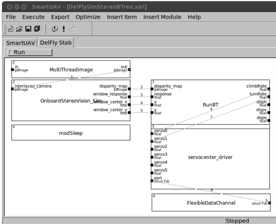
Figure 3-3: SmartUAV GUI showing an Advanced Flight Management System interaction overview chart for the DelFly fly-through-window task
