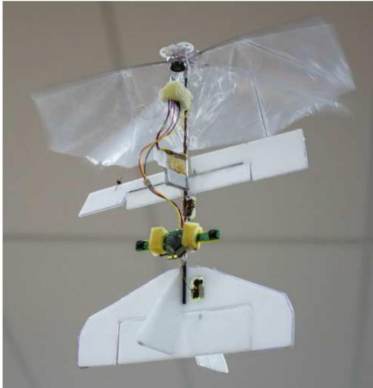
**Figure 3-1:** DeFly Explorer in flight with the camera module in view
