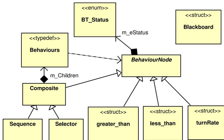
Figure 3-4: UML class diagram of the Behaviour Tree framework for the DelFly
