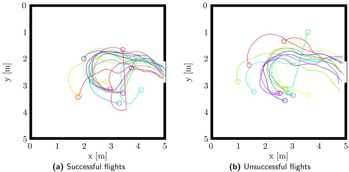
**Figure 6-7:** Flight path tracks of the last 7s of all flights for the genetically optimised behaviour
