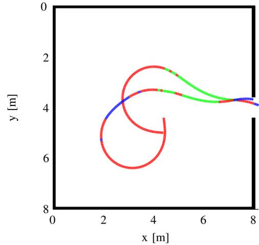
Fig. 11. Path of successful and unsuccessful flight initialisations of DelFly with the genetically optimised behaviour (top-down view). Colours denote different decision modes: Green - window tracking; Blue - default action in low disparity; Red - wall avoidance
