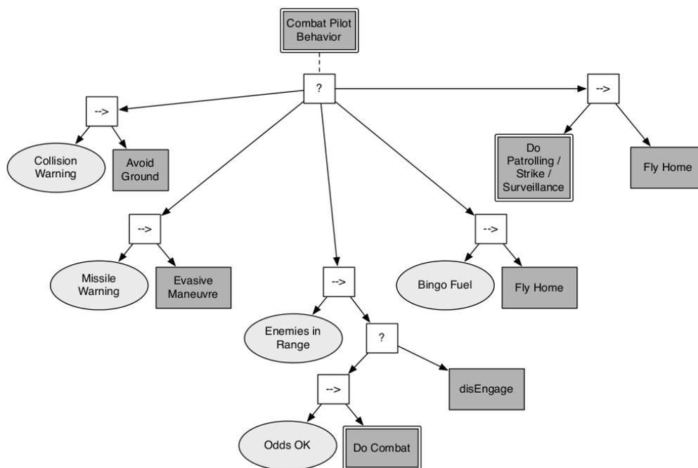
**Figure 2-4:** Example BT defining the behaviour for combat UAV (Ögren, 2012)
