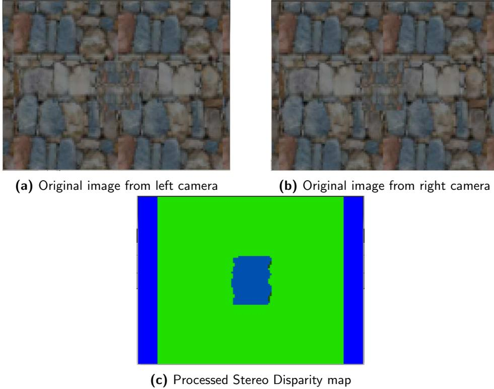
**Figure 3-2:** Original images from left and right camera as well as the resultant disparity map stereo image produced when DelFly aimed at a window in a wall from  $4m$  distance
