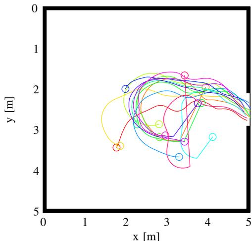
Fig. 18. Flight path tracks of the last 7s of all successful flights for the genetically optimised behaviour. Circle represents start of path
