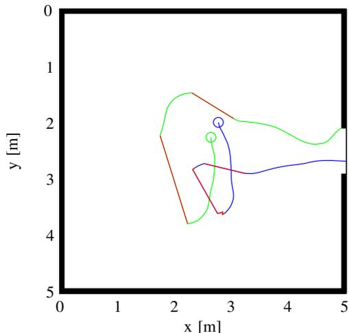
Fig. 17. Flight path tracks showing one complete successful (blue) and unsuccessful (green) flight for the genetically optimised behaviour. Circle represents start location of test. Red track shows area where tracking system lost lock of the DelFly
