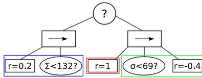
Fig. 9. Graphical depiction of genetically optimised BT. Colours highlight different phases of the flight  $x$  is the position of the centre of the window in frame,  $\sigma$  is window response value,  $\Sigma$  is sum of disparity and  $\Delta$  is the horizontal difference in disparity
