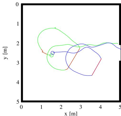
Fig. 20. Flight path tracks showing one complete successful (blue) and unsuccessful (green) flight for the genetically optimised behaviour. Circle represents start location of test. Red track shows area where tracking system lost lock of the DelFly
