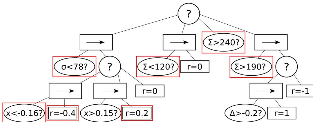
**Figure 6-2:** Graphical depiction of user-defined BT after modification for real world flight. Red boxes highlight updated nodes.  $x$  is the position of the centre of the window in frame,  $\sigma$  is window response value,  $\Sigma$  is sum of disparity and  $\Delta$  is the horizontal difference in disparity
