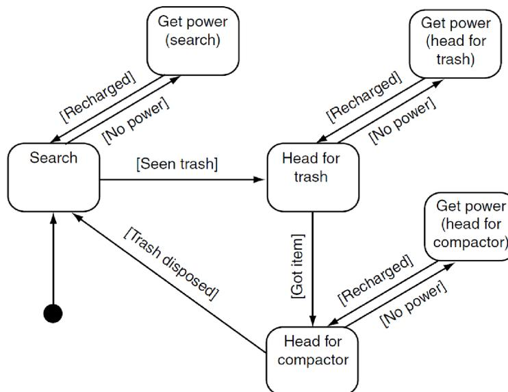
**Figure A-9:** Example of state explosion in FSM (Millington & Funge, 2009)
