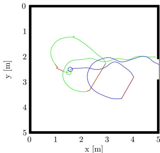
**Figure 6-8:** Flight path tracks showing sample failure and success flight case for the genetically optimised behaviour. Red track shows area where tracking system lost lock of the DelFly
