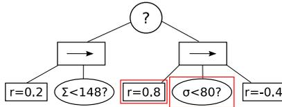
Fig. 14. Graphical depiction of genetically optimised BT after modification for real world flight. Red boxes highlight updated nodes.  $x$  is the position of the centre of the window in frame,  $\sigma$  is window response value,  $\Sigma$  is sum of disparity and  $\Delta$  is the horizontal difference in disparity
