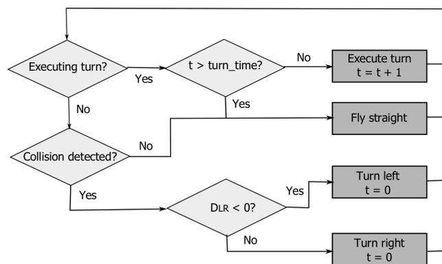
**Figure 2-6:** DelFly obstacle avoidance FSM implementation as defined by de Croon et al. (2012)
