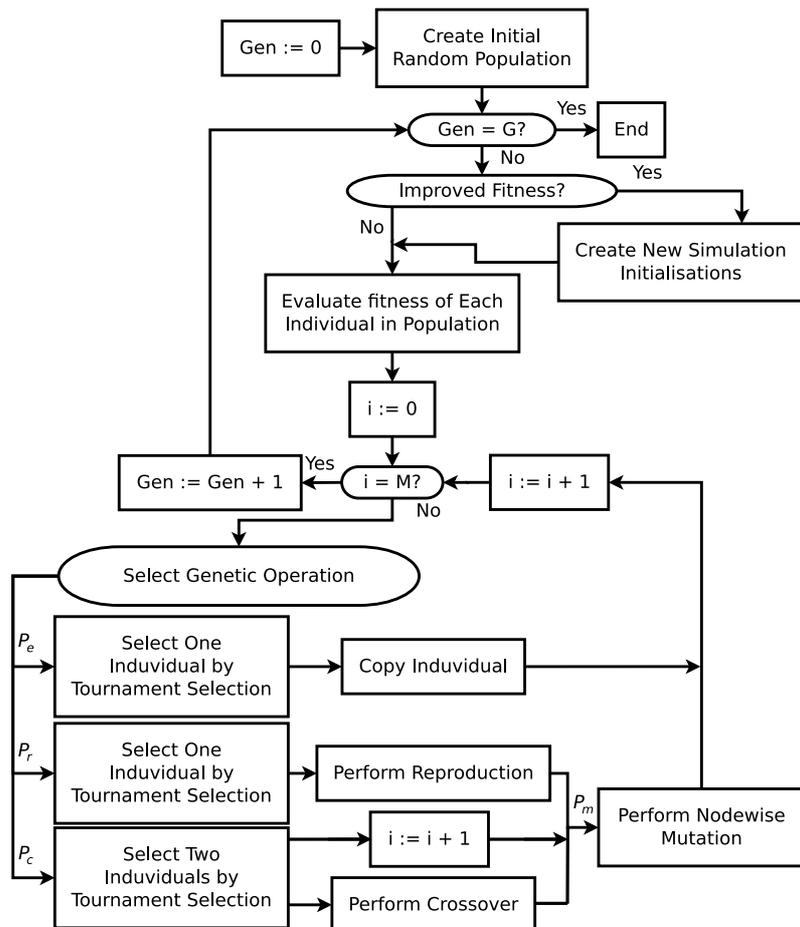
**Figure 4-3:** Flow diagram showing implementation of the Evolutionary Learning architecture for Behaviour Tree evolution
