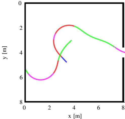
Fig. 3. Path of successful and unsuccessful flight initialisations of DeIFly with the user-defined behaviour (top-down view). Colours denote different decision modes: Green - window tracking; Blue - default action in low disparity; Red - wall avoidance; Magenta - action hold
