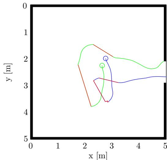
**Figure 6-6:** Flight path tracks showing a sample failure and success flight case for the user defined behaviour. Red track shows area where tracking system lost lock of the DeIFly
