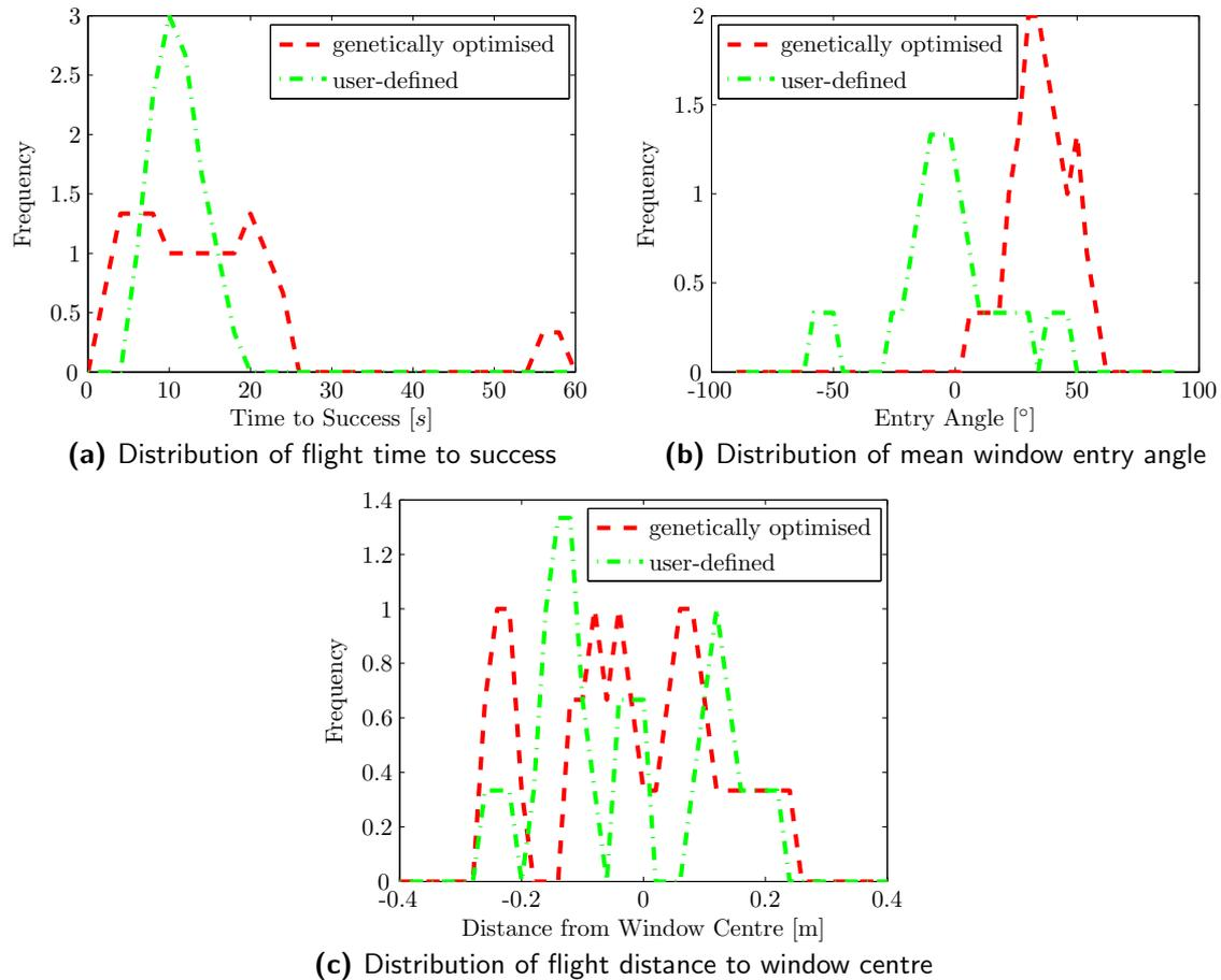
**Figure 6-4:** Distribution of secondary performance parameters from flight test
