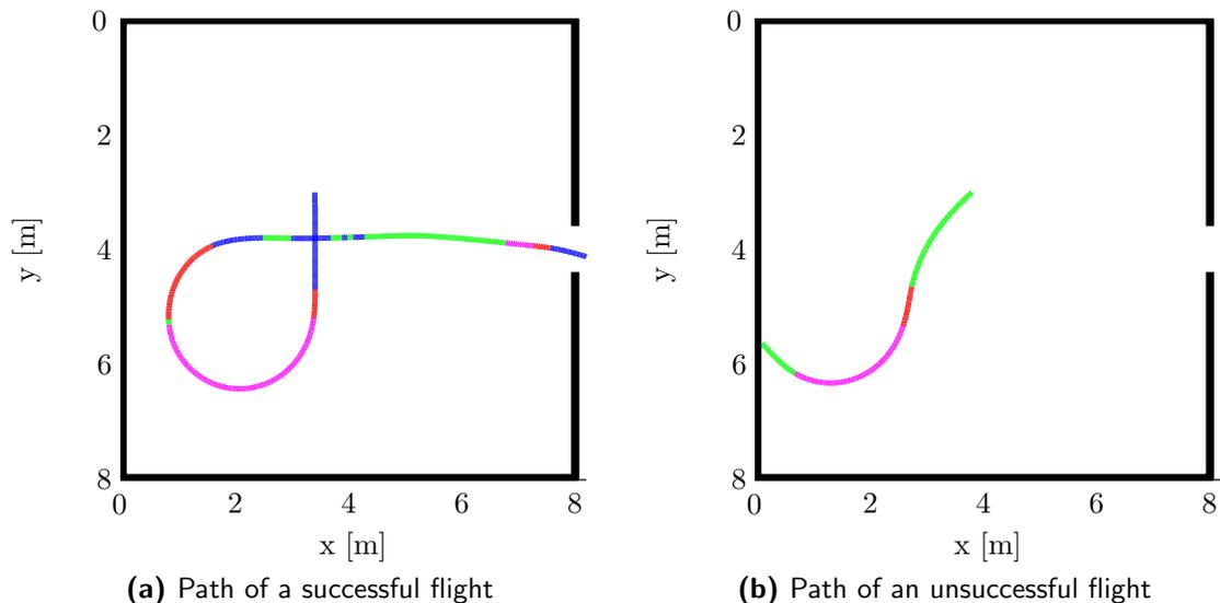
**Figure 5-5:** Path of two flight initialisations of DelFly with the user-defined behaviour (top-down view). Colours denote different decision modes: Green - window tracking; Blue - default action in low disparity; Red - wall avoidance; Magenta - action hold
