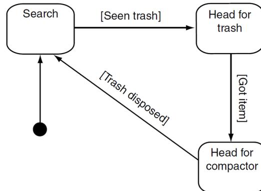
**Figure A-8:** Example of typical finite state machine (Millington & Funge, 2009)
