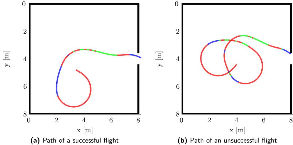
**Figure 5-11:** Path of two flight initialisations of DelFly with the genetically optimised behaviour (top-down view). Colours denote different decision modes: Green - window tracking; Blue - default action in low disparity; Red - wall avoidance
