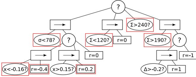
Fig. 13. Graphical depiction of user-defined BT after modification for real world flight. Red boxes highlight updated nodes.  $x$  is the position of the centre of the window in frame,  $\sigma$  is window response value,  $\Sigma$  is sum of disparity and  $\Delta$  is the horizontal difference in disparity
