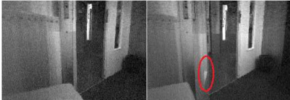
Figure 2-3: Example of perspective distortion. The red circle indicates a window frame in the opened door that is only visible for the right camera
